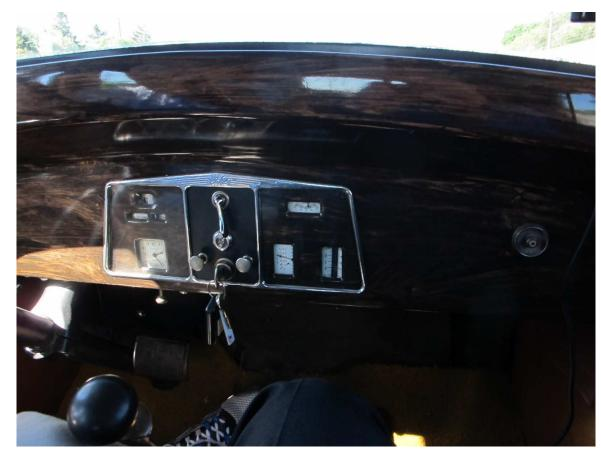
Dashboard includes a rotating drum speedometer, an odometer, a Waltham clock on the left; oil pressure, fuel, and amperes gauges on the right; and headlight, choke, ignition, and spark advance controls in the centre.
