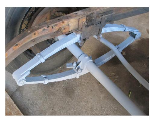
The front axle and springs were re-painted while the engine was removed for rebuilding
